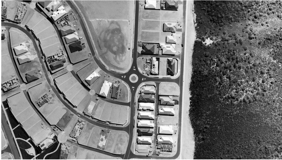
Figure 4. Example of remodelling undulating sand dune terrain into a large earthwork of retaining walls (demarcated by their shadows) and perfectly flat buildings lots to facilitate rapid suburban expansion in Perth, Australia. 2012.
