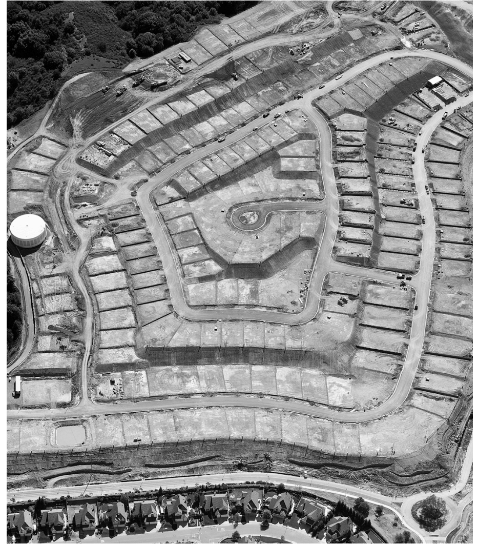
Figure 3. Example of site preparation for new suburban development at Hayward, California.
